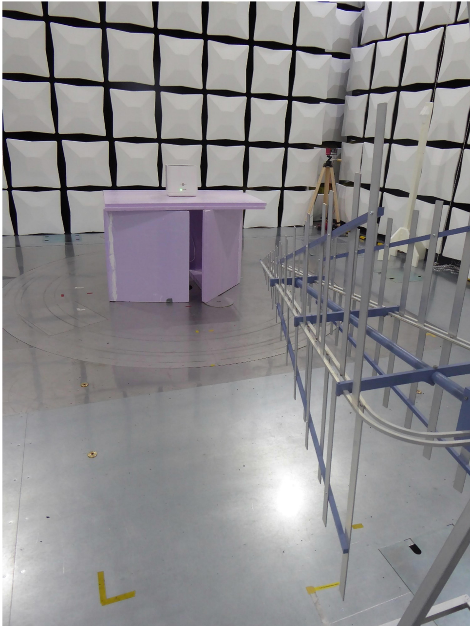
Test setup semi-anechoic chamber M276, 30 MHz - 1 GHz
