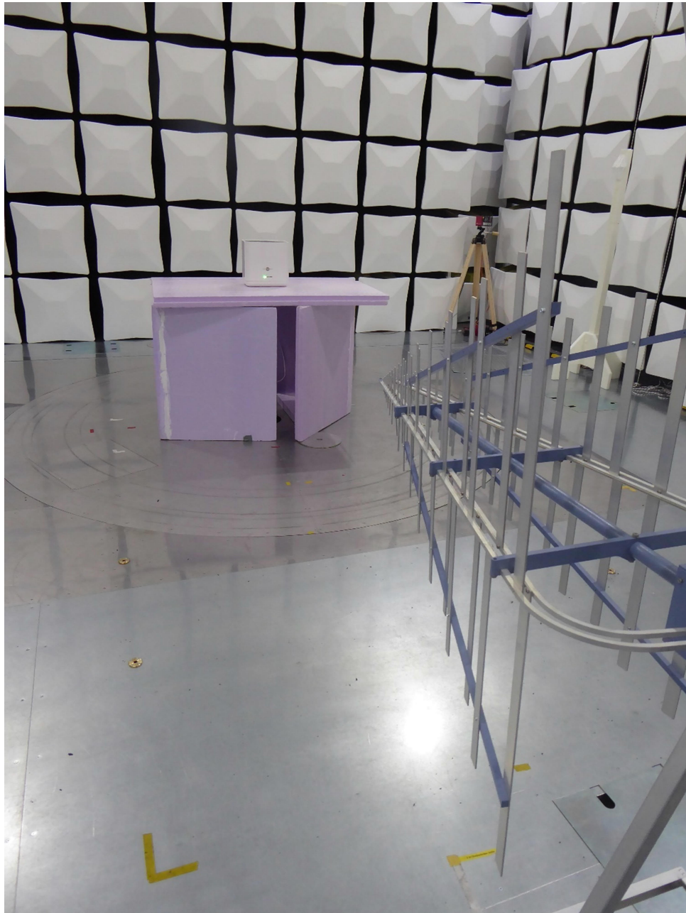
Test setup semi-anechoic chamber M276, 30 MHz - 1 GHz
