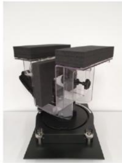
Figure 4.4 Mounting Device for Hand-held Devices and Laptop / Body-Worn Devices
