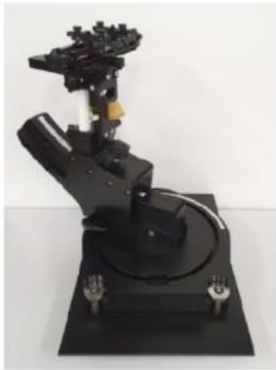
Figure 4.4 Mounting Device for Hand-held Devices and Laptop / Body-Worn Devices
