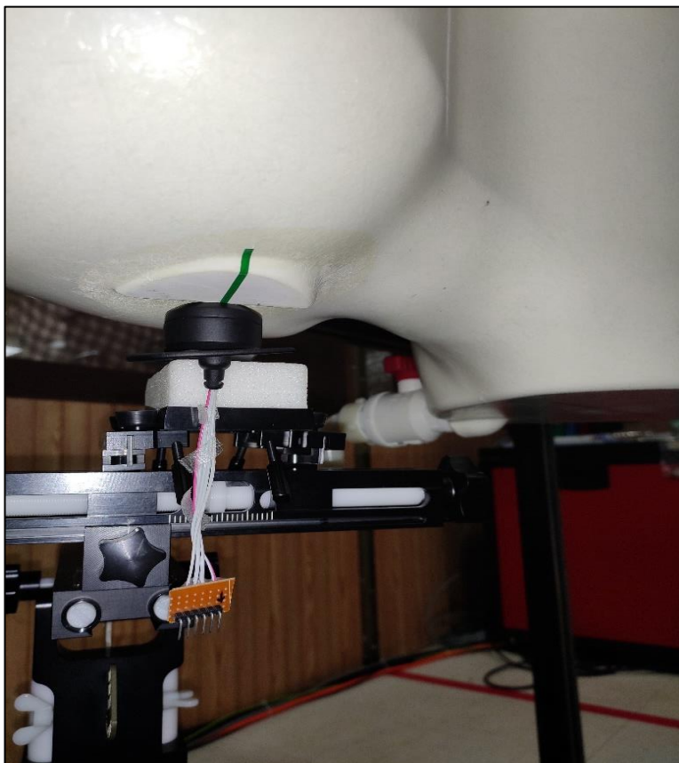
Photo 2 : EUT kept in Cheek position with the Left head phantom
