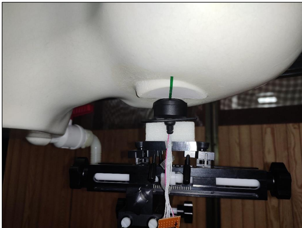
Photo 1 : EUT kept in Cheek position with the Right head phantom
