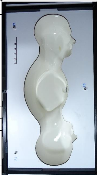
Figure 5: Twin SAM Phantom
