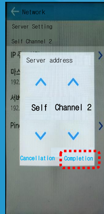
Slave address Setting / Save by tapping Complete tab
