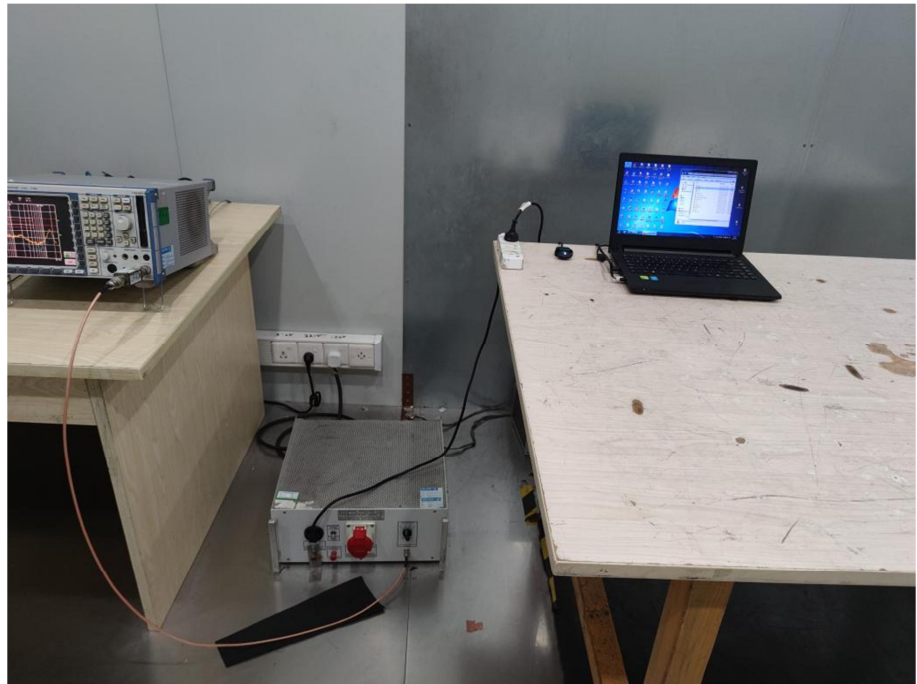
Conducted Emission Test Setup
