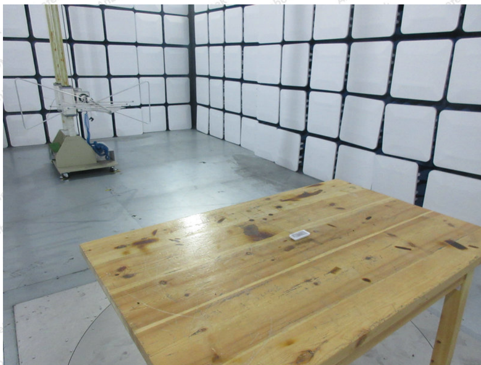
Photo of Radiation Emission Test
