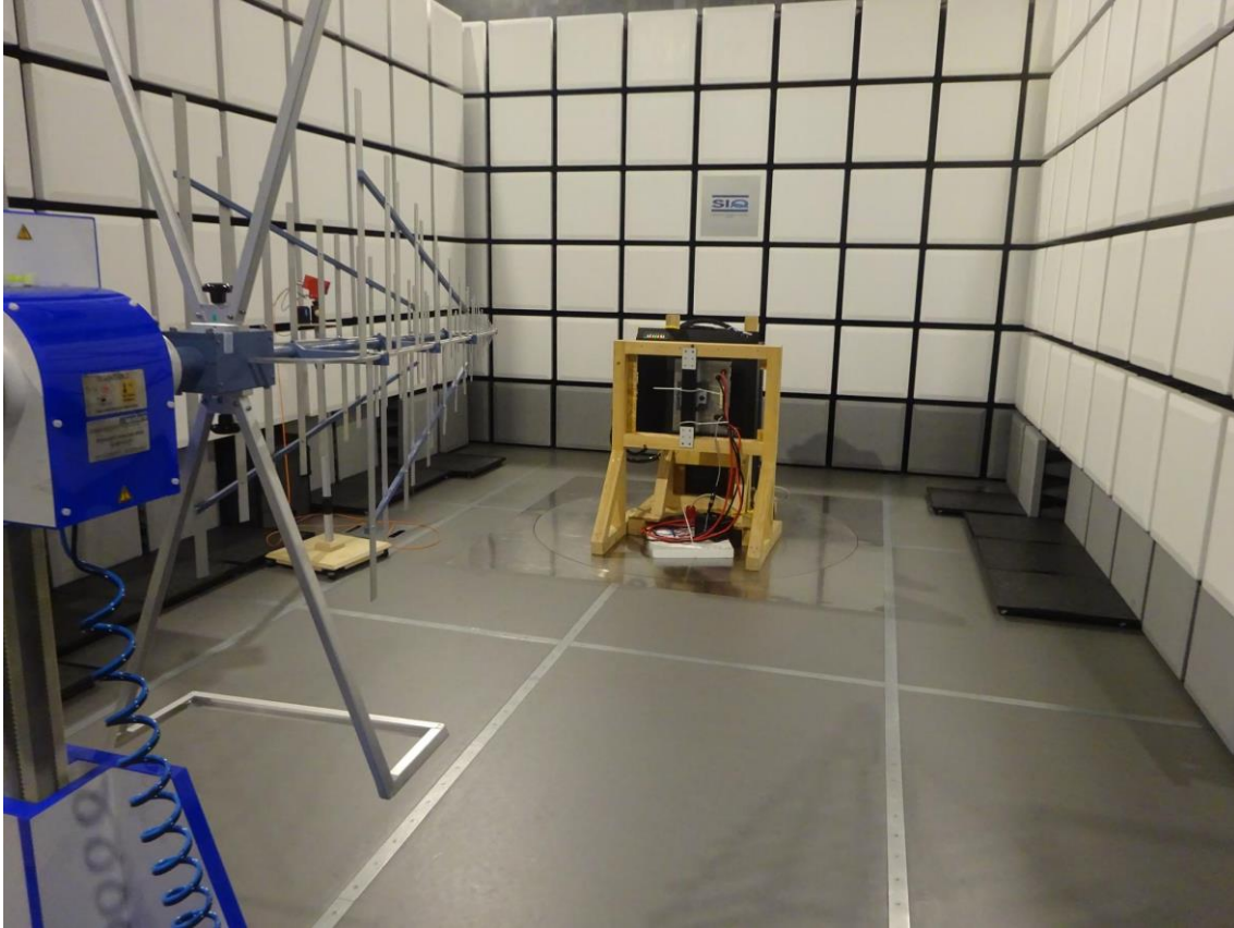
Figure 3: Radiated emissions from 30 MHz – 1000 MHz Landscape mode
