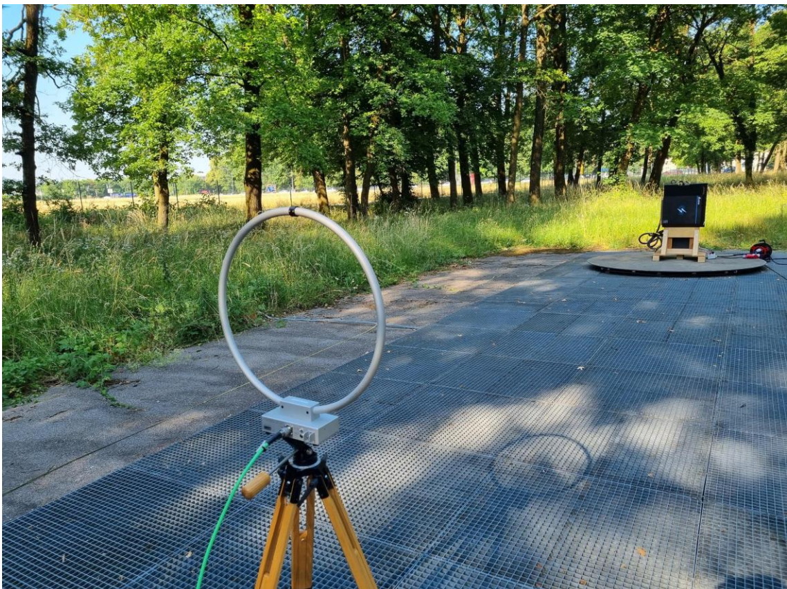
Figure 10: Radiated emissions on OATS
