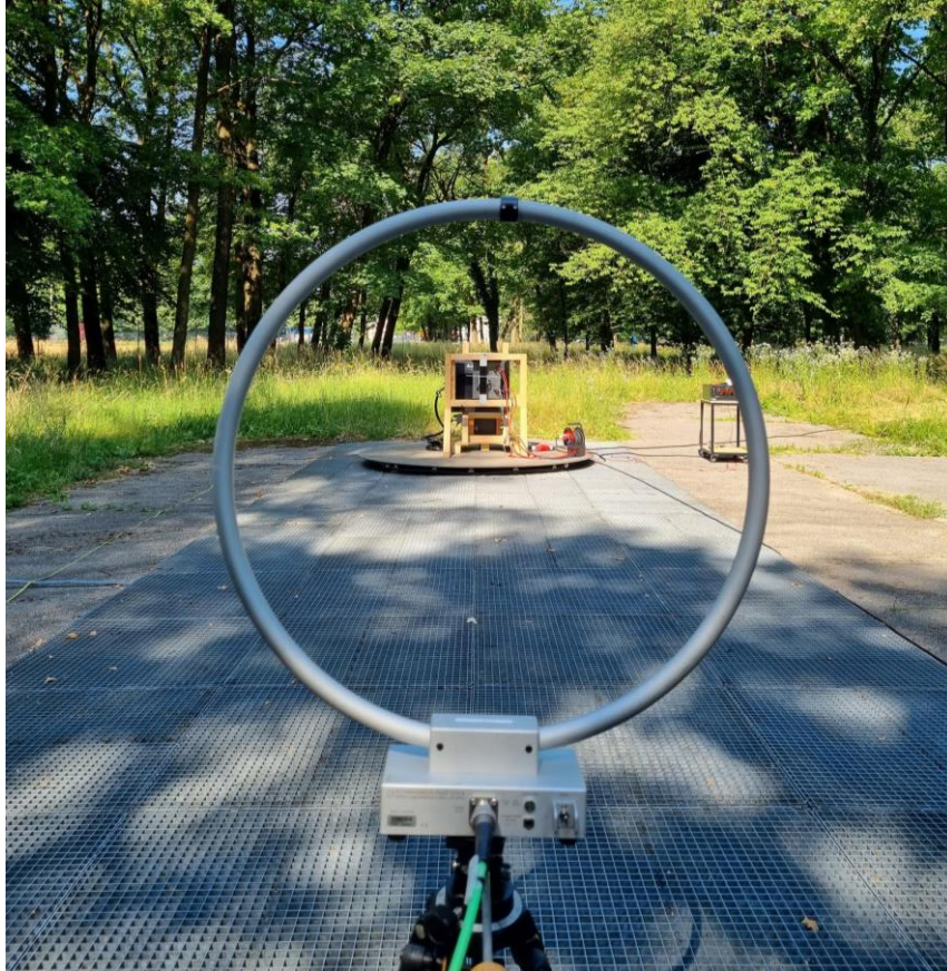
Figure 11: Radiated emissions on OATS
