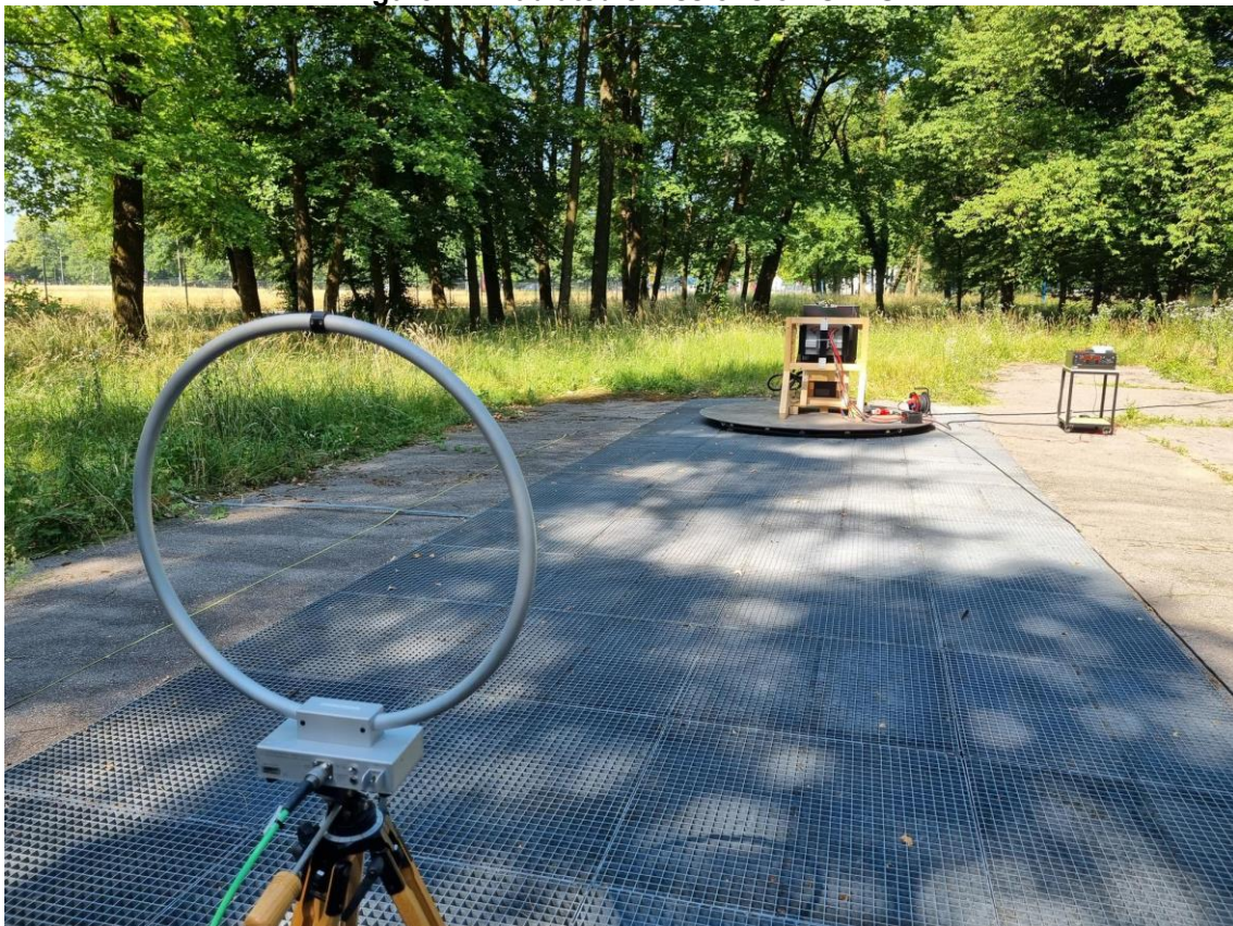
Figure 12: Radiated emissions on OATS
