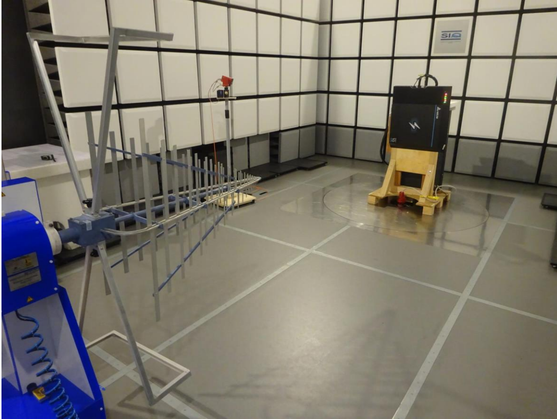
Figure 7: Radiated emissions from 30 MHz – 1000 MHz Portrait mode
