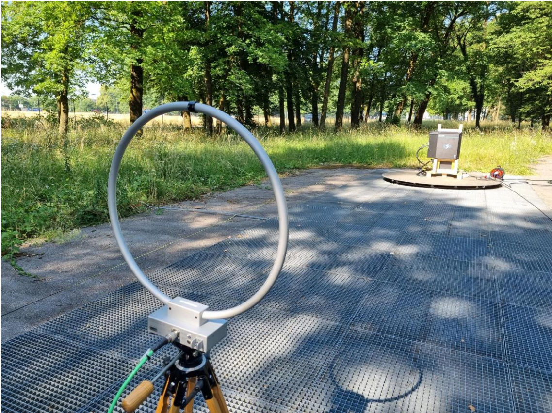
Figure 9: Radiated emissions on OATS
