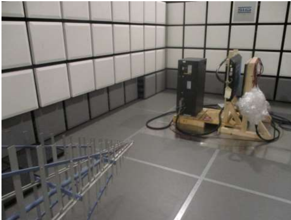
Figure 3: Radiated emission test 30 MHz – 1000 MHz: measurement in SAC with 3 m measurement distance
