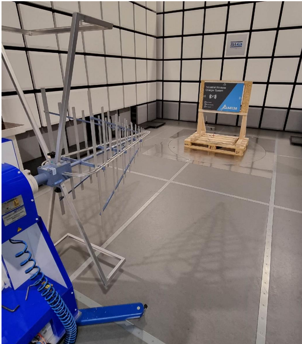
Figure 2: Radiated measurements 30 MHz-1000 MHz
