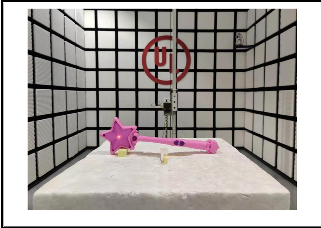
RADIATED RF MEASUREMENT SETUP (Above 1G – Z axis)
