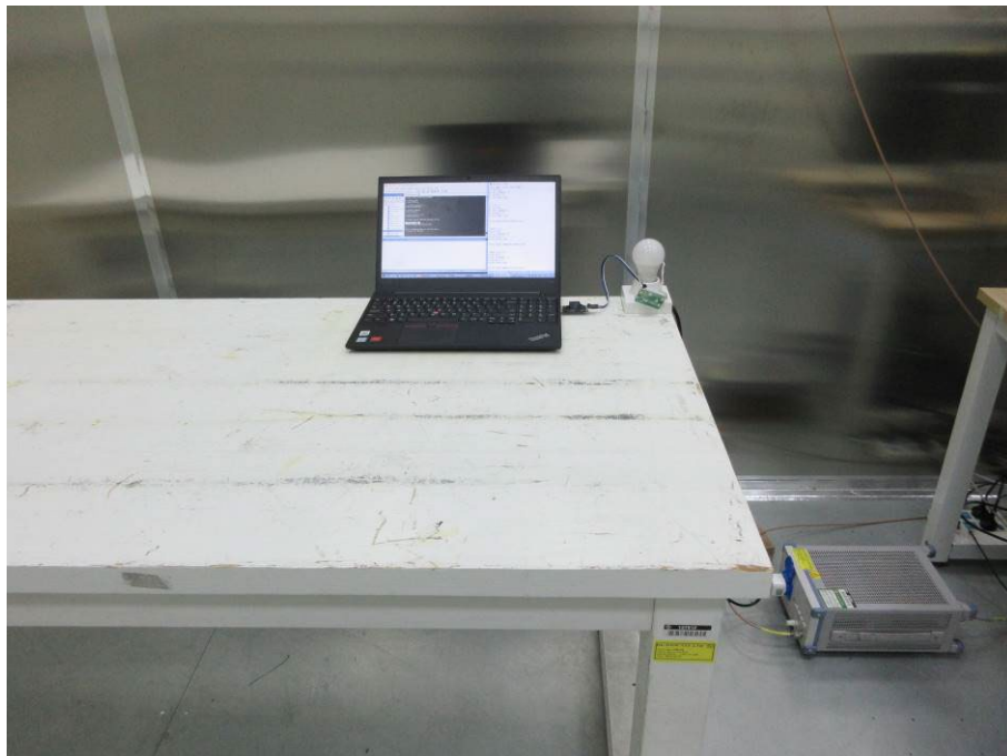
POWERLINE CONDUCTED EMISSIONS MEASUREMENT SETUP
