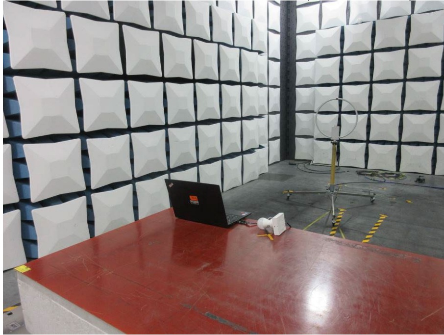
RADIATED RF MEASUREMENT SETUP (9kHz ~ 30 MHz)
