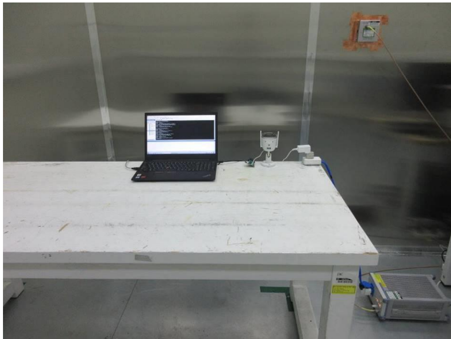
POWERLINE CONDUCTED EMISSIONS MEASUREMENT SETUP
