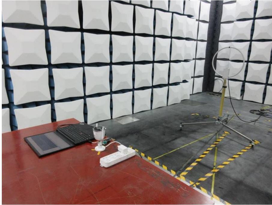
RADIATED RF MEASUREMENT SETUP (9kHz ~ 30 MHz)
