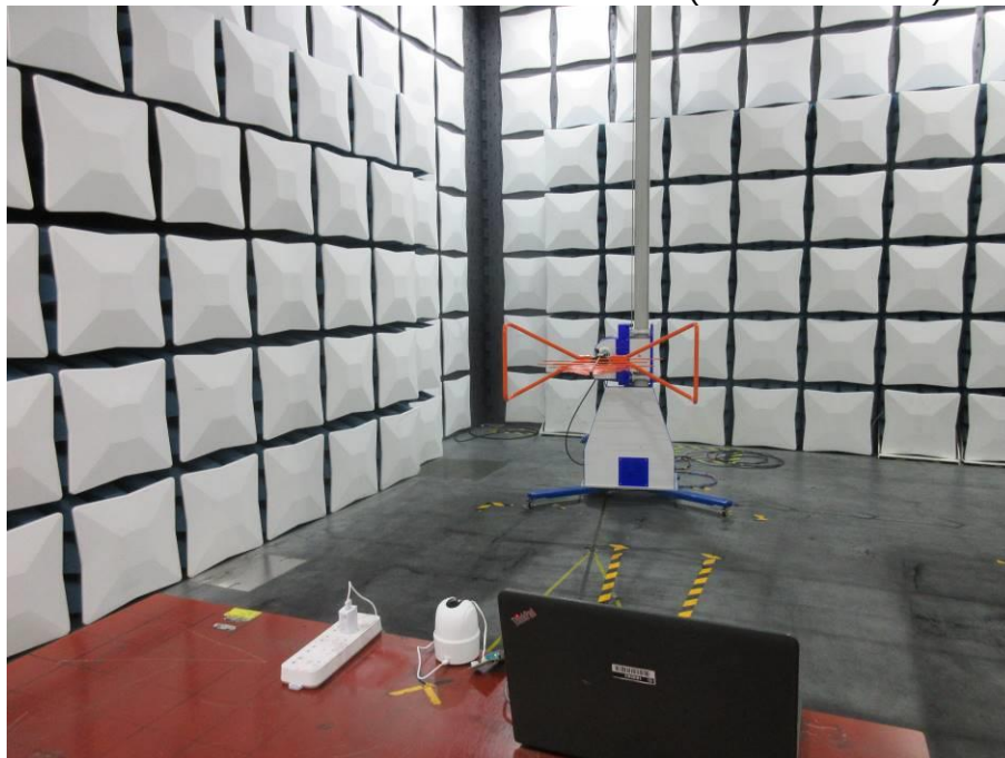
RADIATED RF MEASUREMENT SETUP (30MHz ~ 1 GHz)
