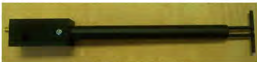
Figure 1 – MVG COMOSAR Validation Dipole
