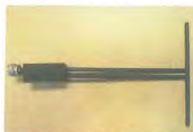
Figure 1 – MVG COMOSAR Validation Dipole
