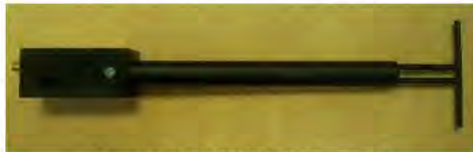
Figure 1 – MVG COMOSAR Validation Dipole
