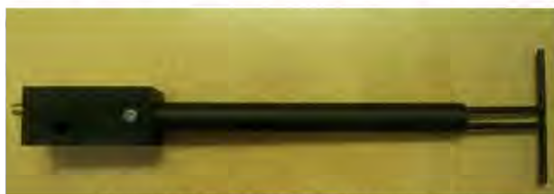
Figure 1 – MVG COMOSAR Validation Dipole
