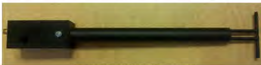
Figure 1 – MVG COMOSAR Validation Dipole
