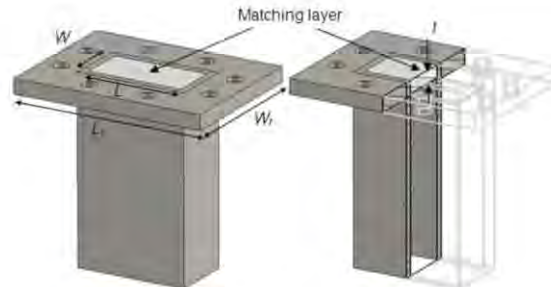
Figure 1: Validation Waveguide Dimensions
