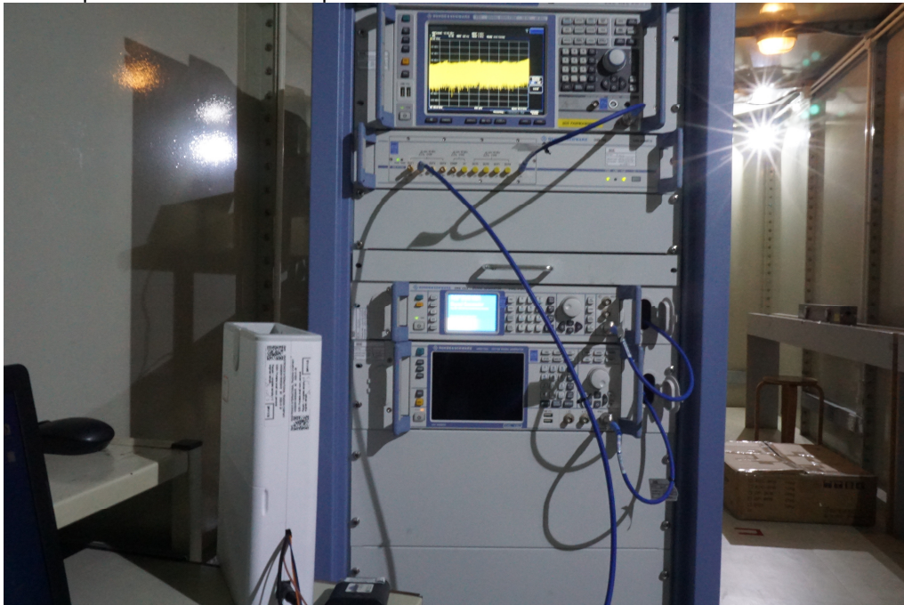
Conducted Spurious Test Test Setup
