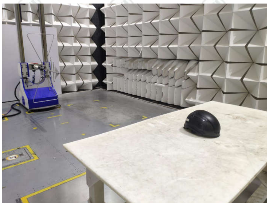
Radiated spurious emission Test Setup-2(Below 1GHz)
