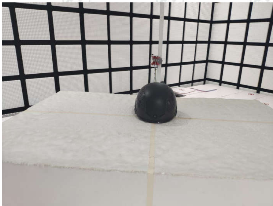
Radiated spurious emission Test Setup-3(Above 1GHz)
