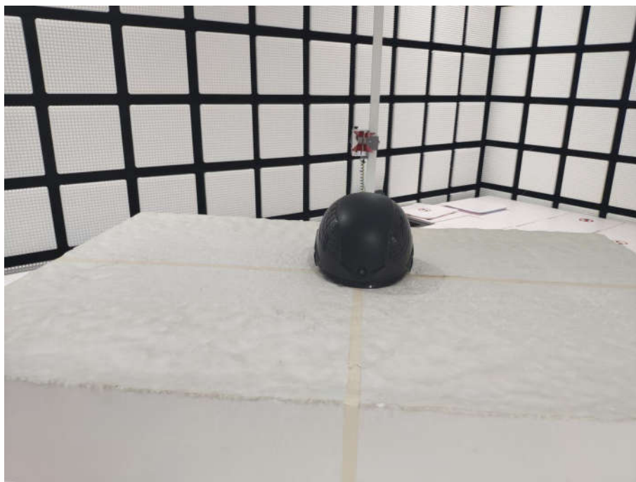
Radiated spurious emission Test Setup-3(Above 1GHz)
