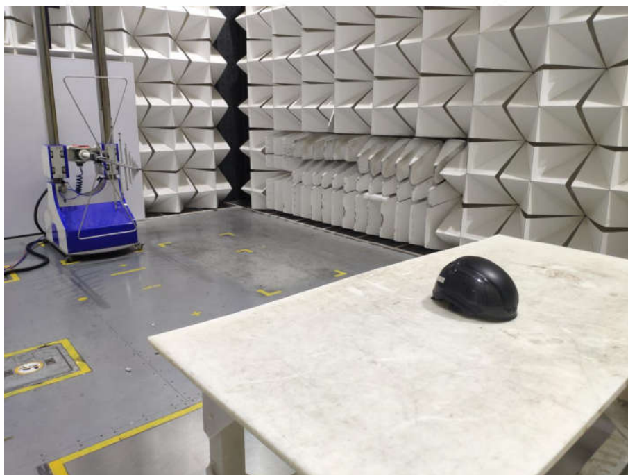
Radiated spurious emission Test Setup-2(Below 1GHz)
