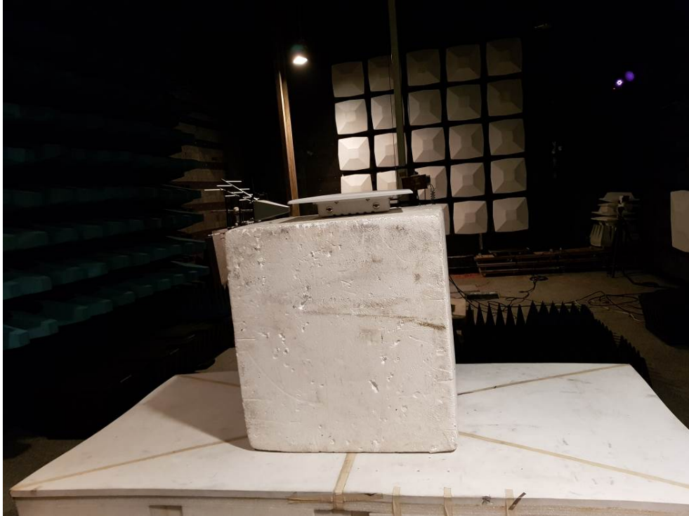
Photograph – Radiated Emission Test Set up_Above 1GHz
