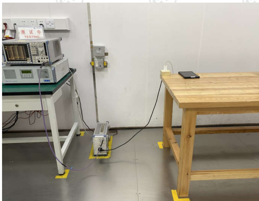
Conducted Emissions Test Setup
