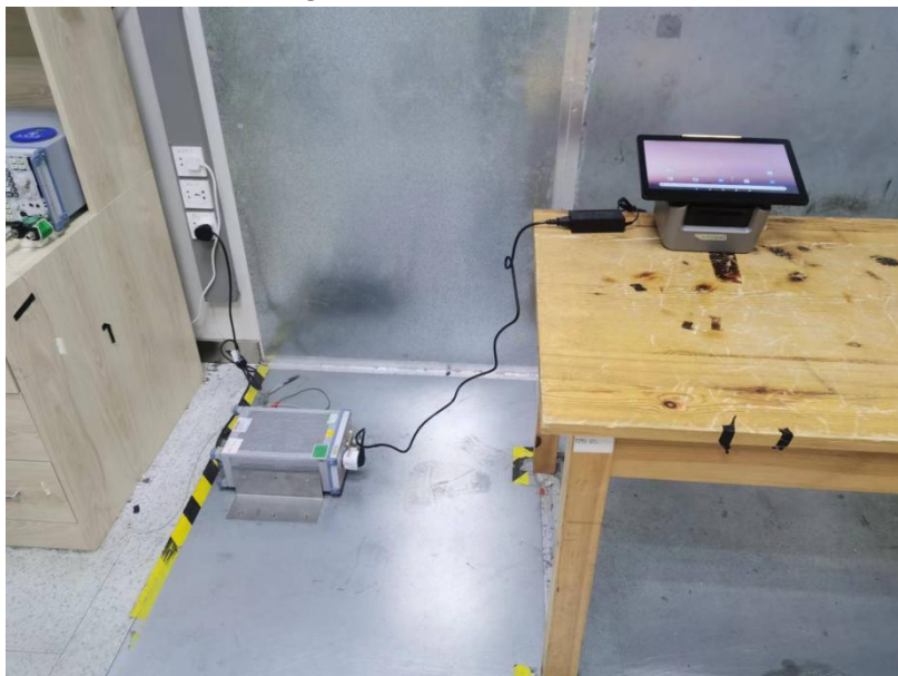
Radiated Spurious Emissions From 30MHz-1000MHz
