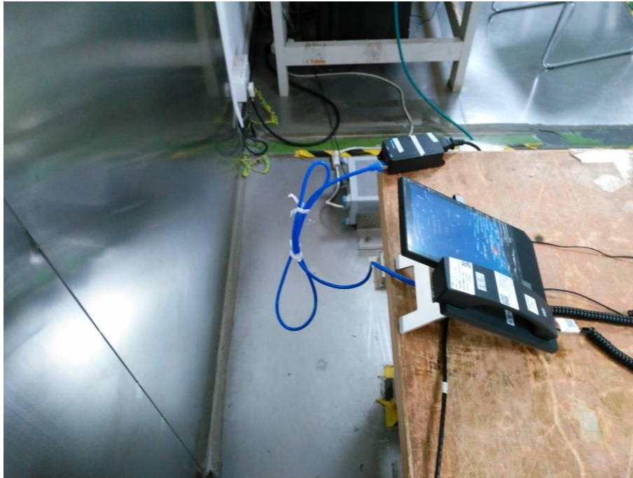
Conducted Emissions - Side View (Powered by POE)
