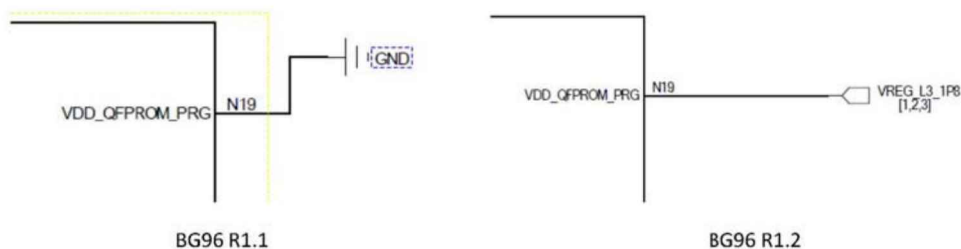
Figure 1: Schematic Designs of BG96 R1.1 and R1.2
