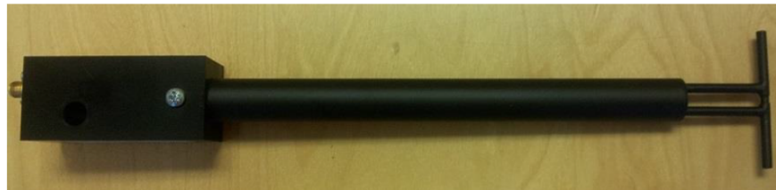
Figure 1 – MVG COMOSAR Validation Dipole
