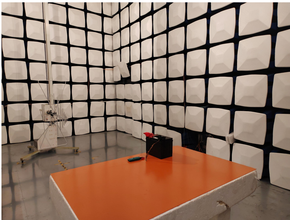
Test Setup Photo(s) of Radiated Emissions Measurement
