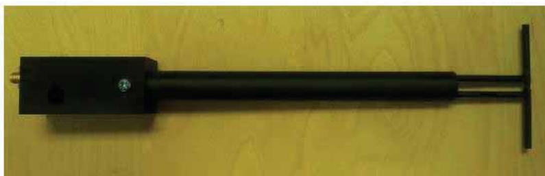
Figure 1 – MVG COMOSAR Validation Dipole
