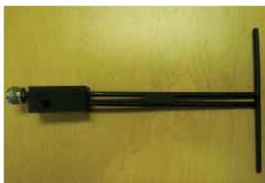
Figure 1 – MVG COMOSAR Validation Dipole
