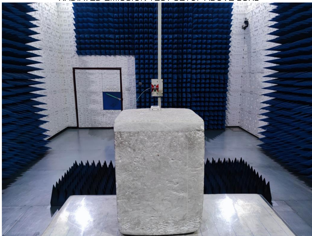
RADIATED EMISSION TEST SETUP ABOVE 1GHz
