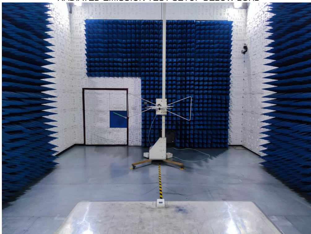
RADIATED EMISSION TEST SETUP ABOVE 1GHz
