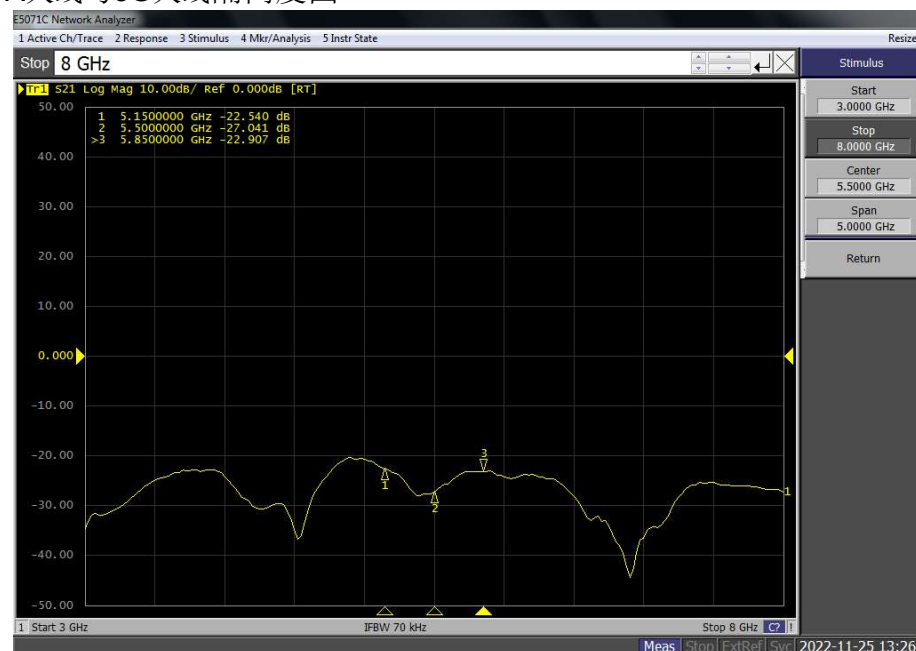
Isolation of antenna A and 5G antenna
