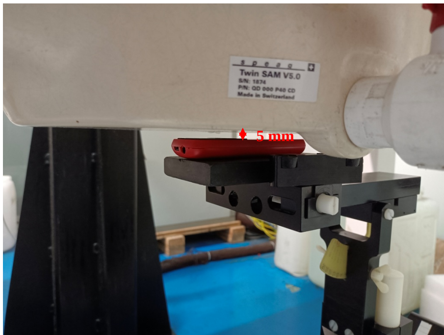
Body (Worn) Front Setup Photo (5mm)
