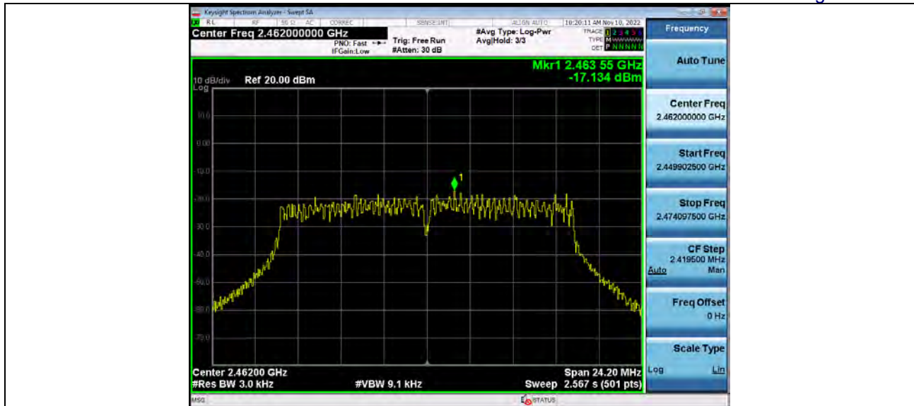
Power Spectral Density 2_4GWiFi_2412_00
