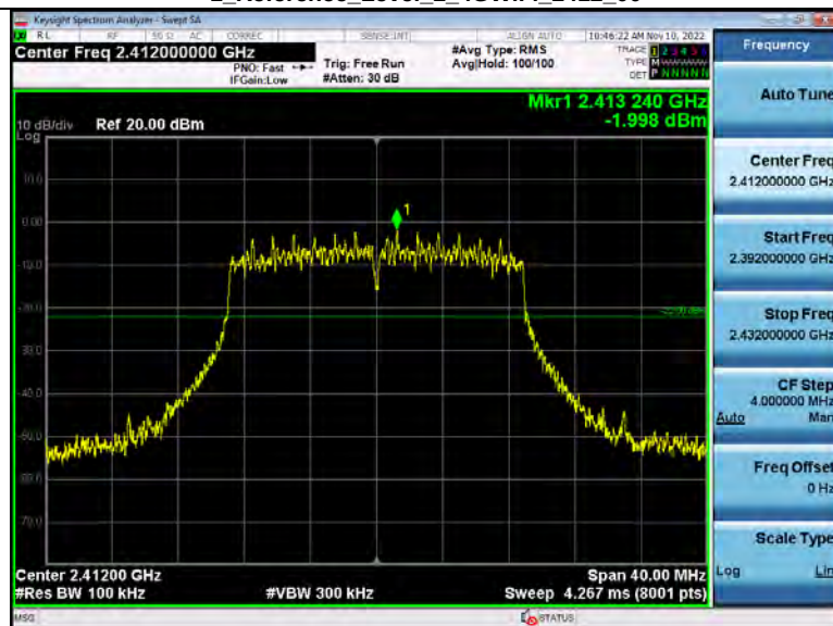
2 Spurious Emission 2 4GWiFi_NVNT_ANT1_802_11n(HT20)_2412_00
