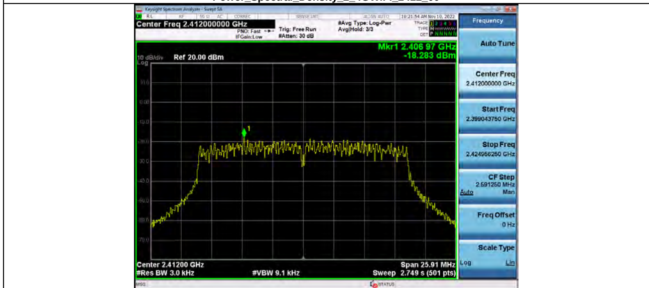
Power Spectral Density 2_4GWiFi_2412_00
