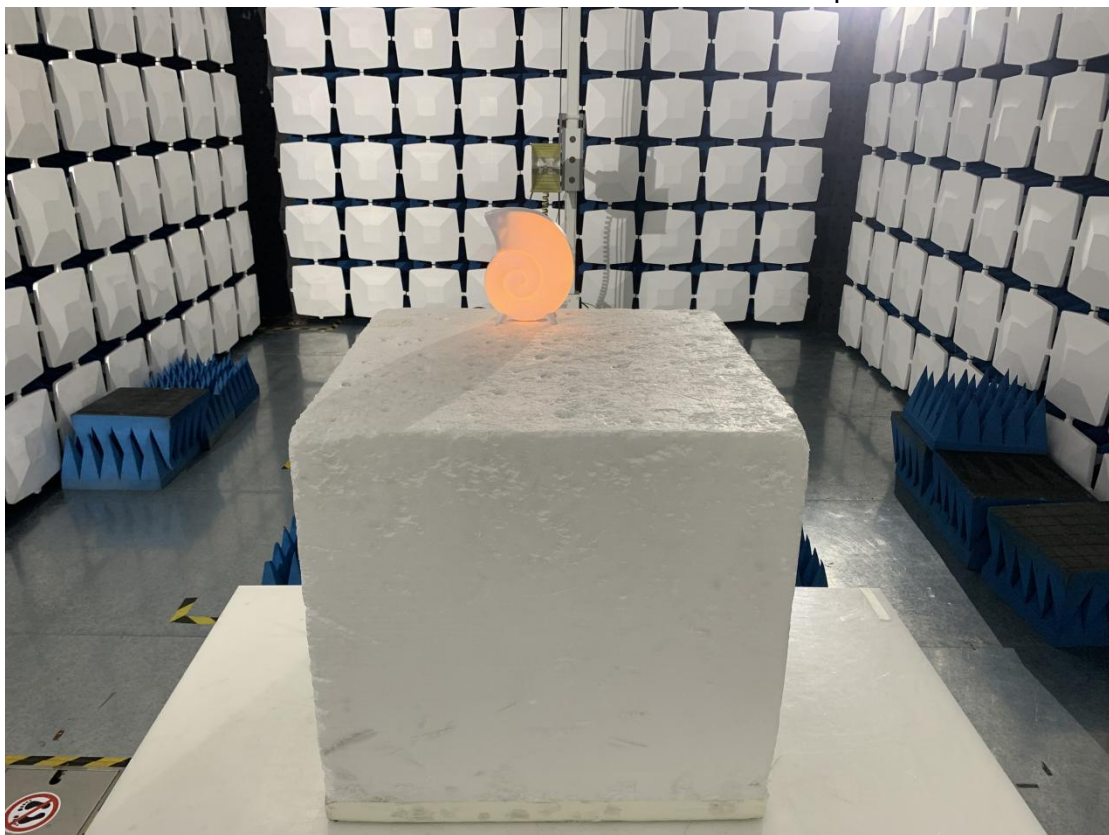
Above 1GHz for radiated emission test setup
