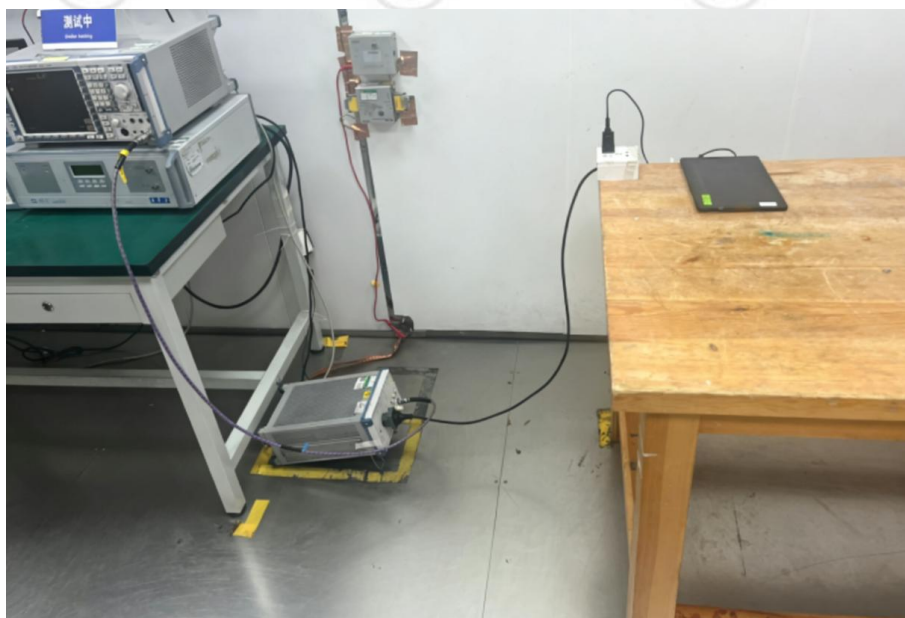
Conducted Emissions Test Setup
