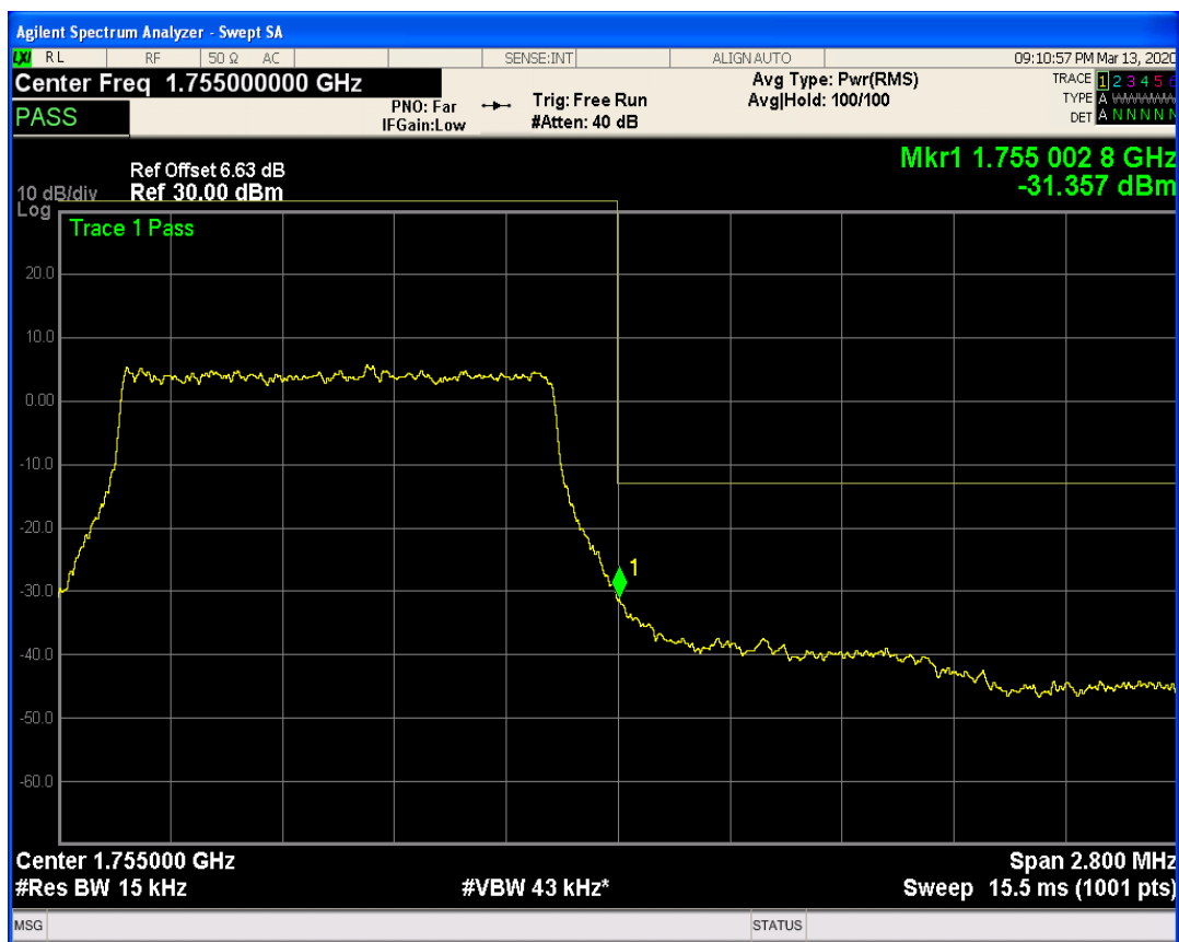
LTE Band4 QPSK BW=3MHz Channel=19965 RB Size=1 Position=#0
