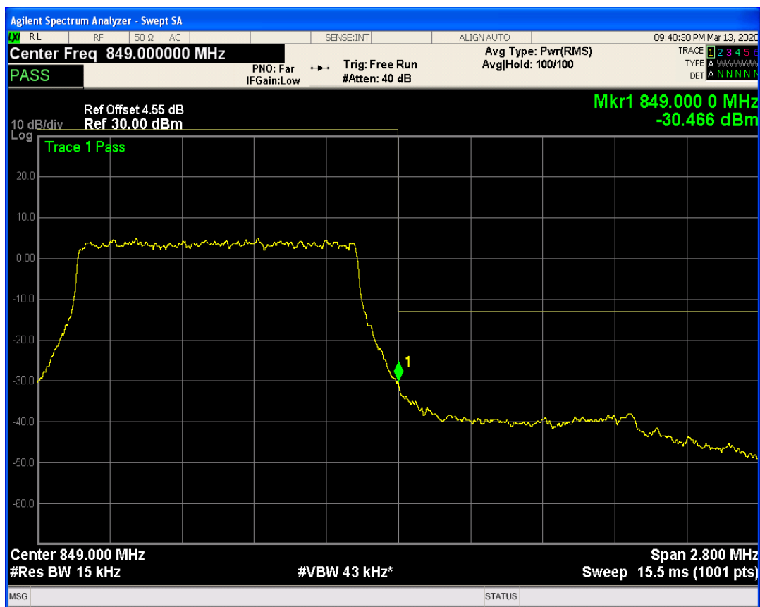
LTE Band5 QPSK BW=3MHz Channel=20415 RB Size=1 Position=#0
