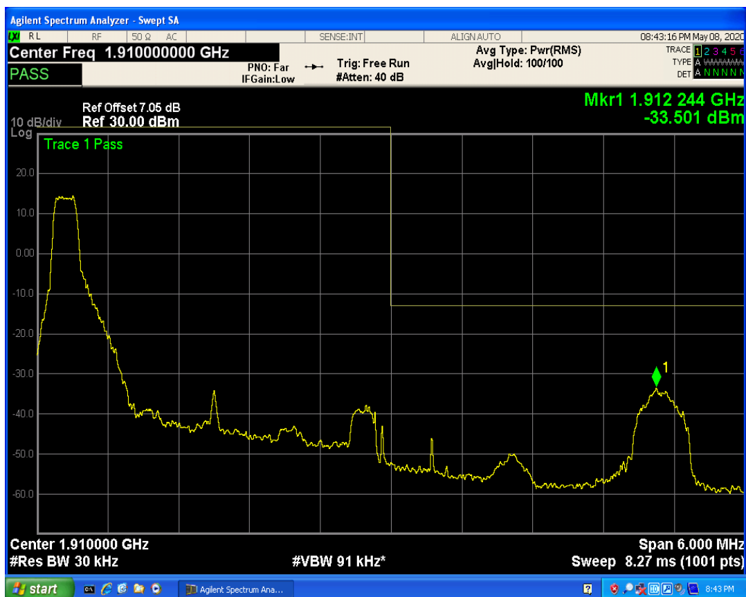
LTE Band2 QAM16 BW=3MHz Channel=19185 RB Size=1 Position=#Max
