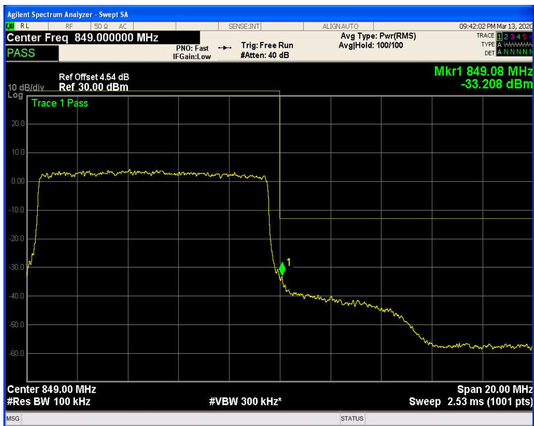
LTE Band5 QPSK BW=10MHz Channel=20600 RB Size=1 Position=#Max
