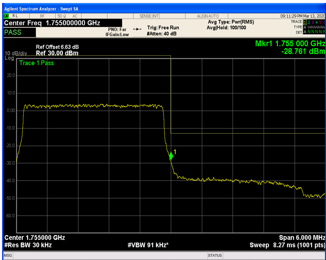
LTE Band4 QPSK BW=5MHz Channel=19975 RB Size=1 Position=#0
