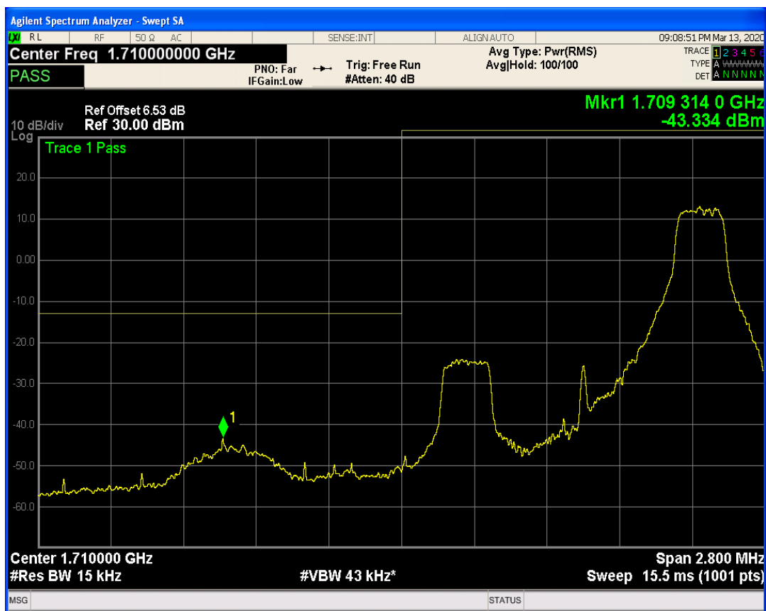
LTE Band4 QPSK BW=1.4MHz Channel=19957 RB Size=6 Position=#0
