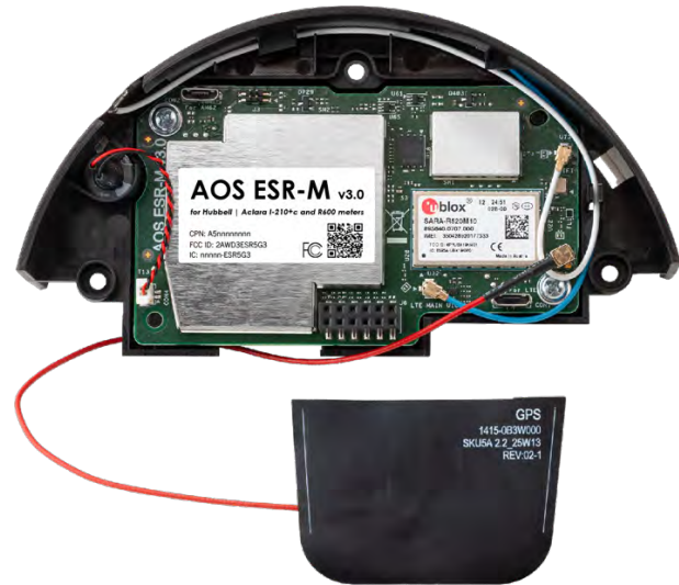
AOS Edge Card for Residential Electricity Meters
