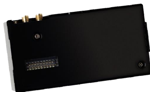
Figure 2 – AOS ESR-M in Enclosure with view of the Meter Interface & Antenna connectors
