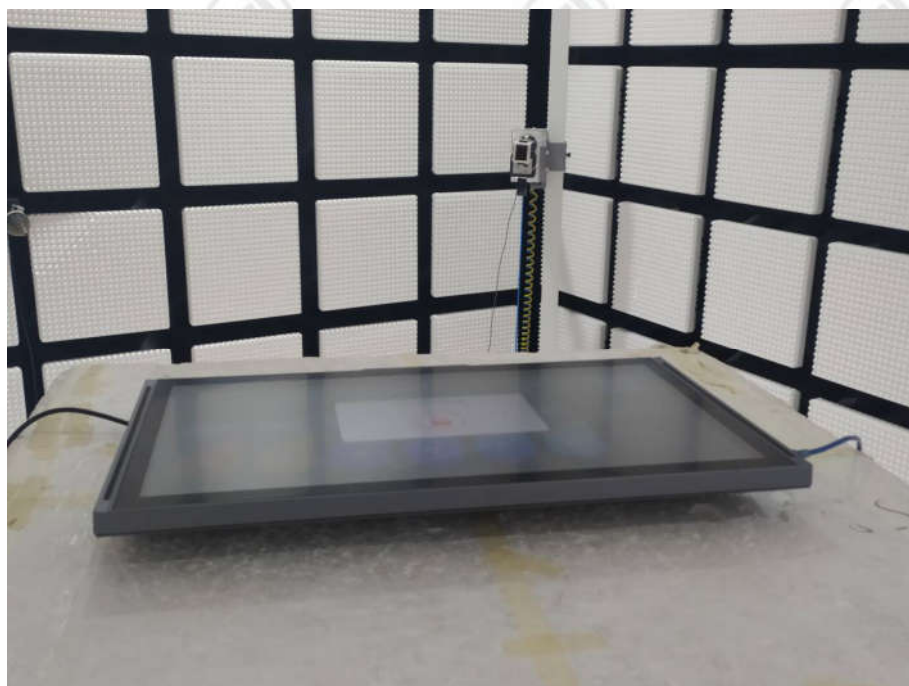
Radiated spurious emission Test Setup-3(Above 18GHz)
