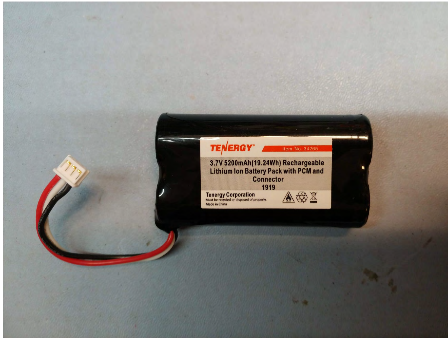
Main Power Battery
