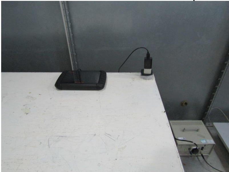
Measurement of Conducted Emission Test Set Up
