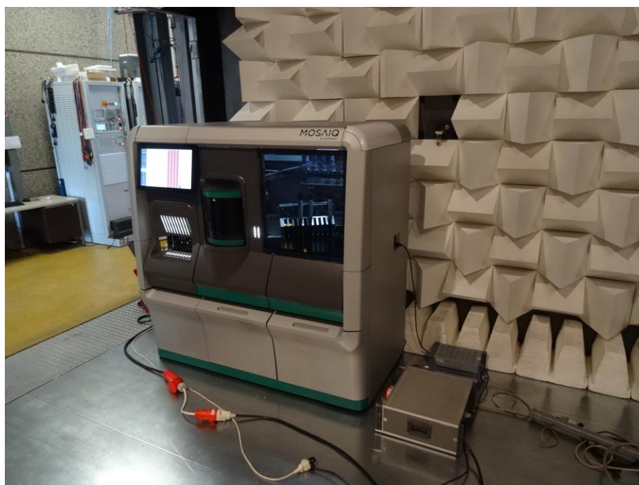
Figure 1 EUT / set up - test module EC (spurious conducted 150 kHz - 30 MHz)
