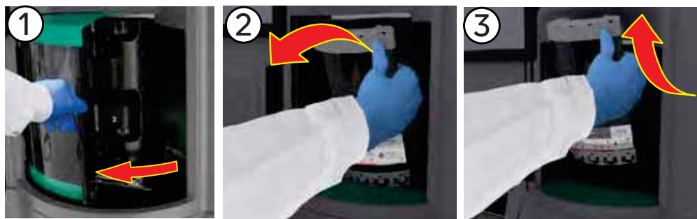
(magazine station door opening and magazine removing)
