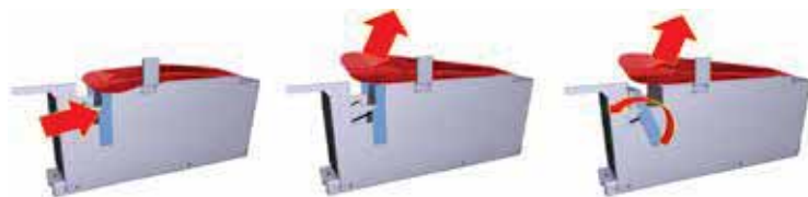
(removing of the solid waste bag)
