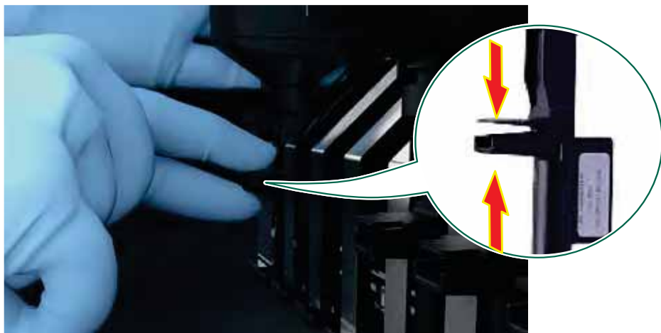
(reagent bottles lock mechanism)
