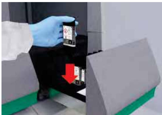
(inserting the buffer and diluent bottles)
