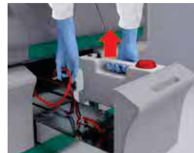
(removing the liquid and solid waste)
