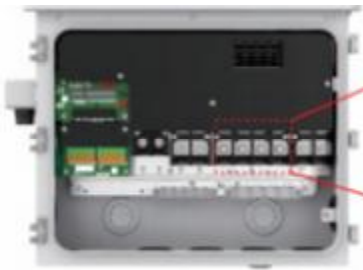
Figure 5. 14 Battery Cable Connection
