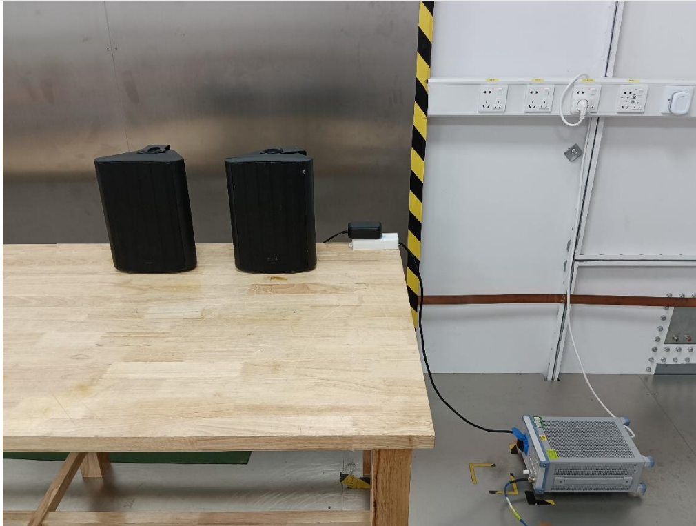
AC Power Line Conducted Emission
