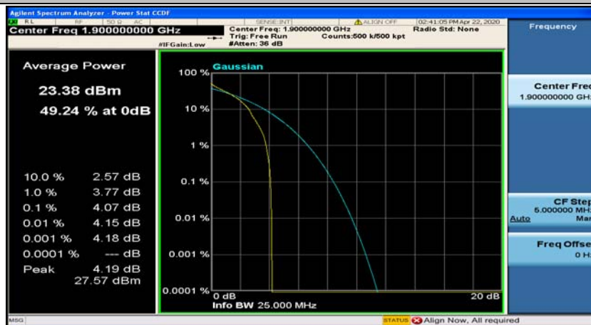
(Channel Bandwidth:20 MHz)_HCH_QPSK_50RB#0
