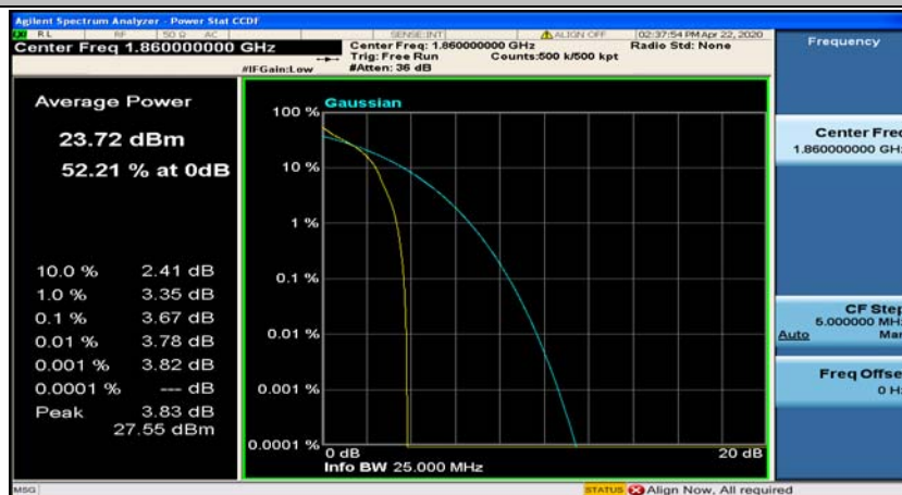
(Channel Bandwidth:20 MHz)_LCH_QPSK_50RB#0
