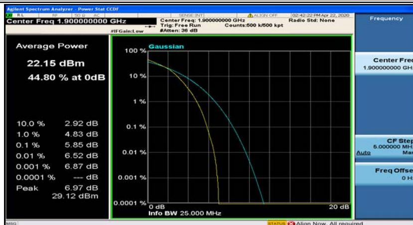
(Channel Bandwidth:20 MHz)_HCH_16QAM_100RB#0
