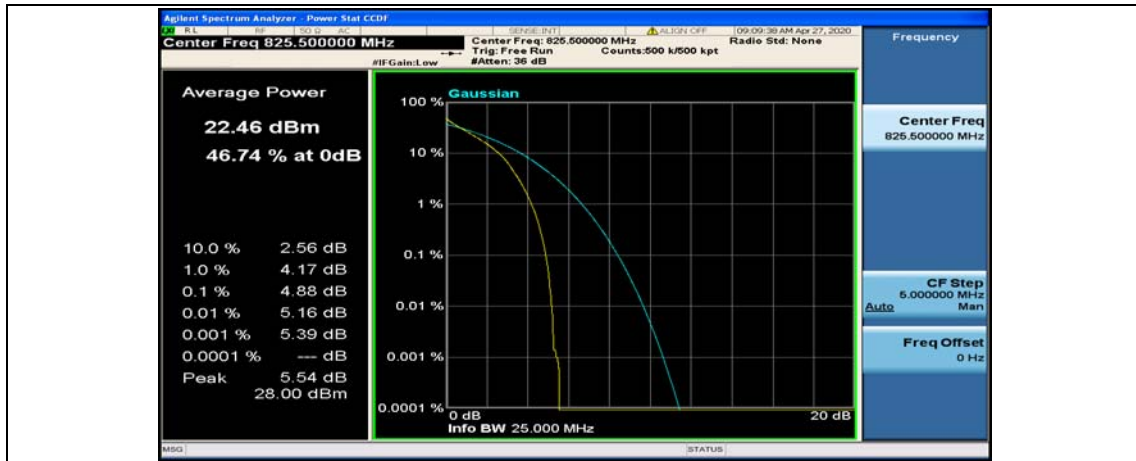
(Channel Bandwidth: 3 MHz)_MCH_QPSK_1RB#0
