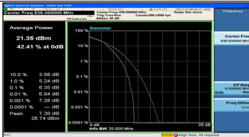
(Channel Bandwidth: 3 MHz)_MCH_16QAM_15RB#0
