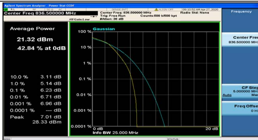
(Channel Bandwidth: 3 MHz)_MCH_16QAM_8RB#7
