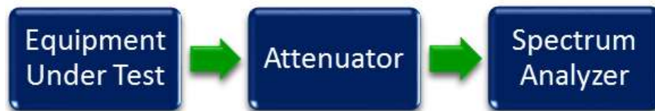
Figure 3. Occupied Bandwidth Test Setup
