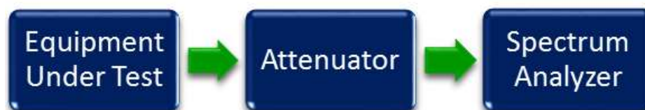
Figure 3. Occupied Bandwidth Test Setup
