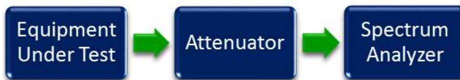
Figure 3. Occupied Bandwidth Test Setup
