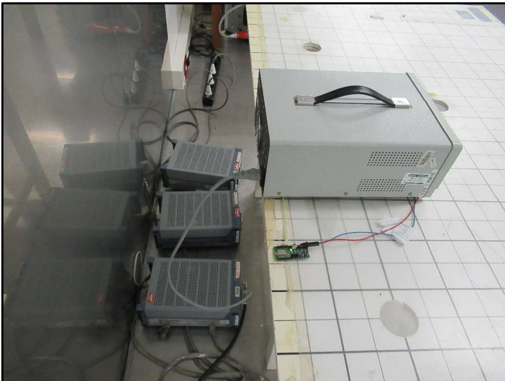
Photo 17 AC Conducted Emissions Test Setup- with DC Power Supply
