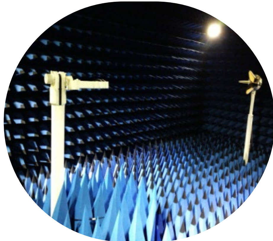
7*4*3M Microwave anechoic chamber
